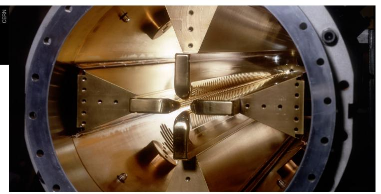
A radio-frequency quadrupole at CERN. The precision-machined modulated electrodes ("vanes") are shaped to first bunch the dcbeam from the ion source and then provide simultaneous acceleration and focusing of the beam
