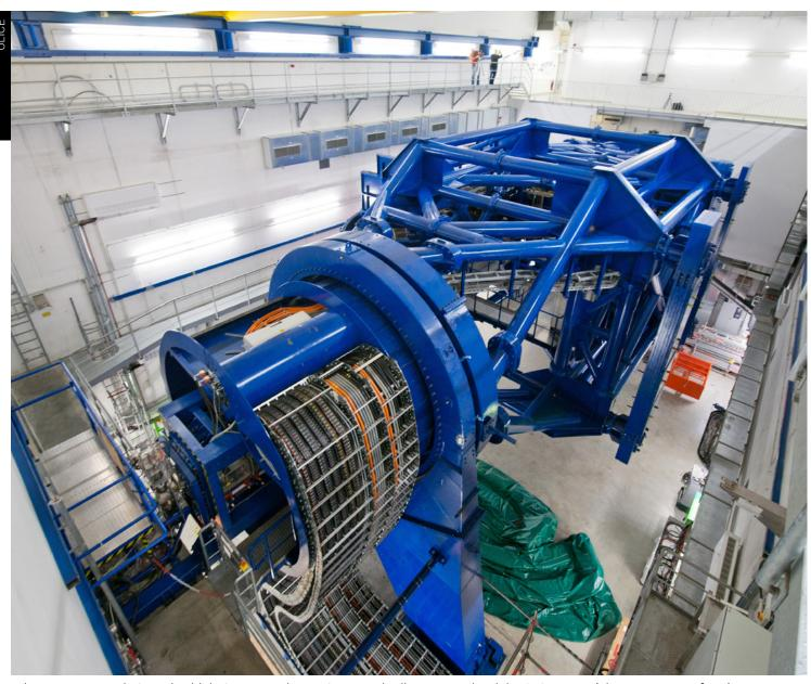
The gantry at HIT is 3 stories high, 25 metres long, 13 metres in diametre and weighs 670 tonnes (photo courtesy of HIT)
